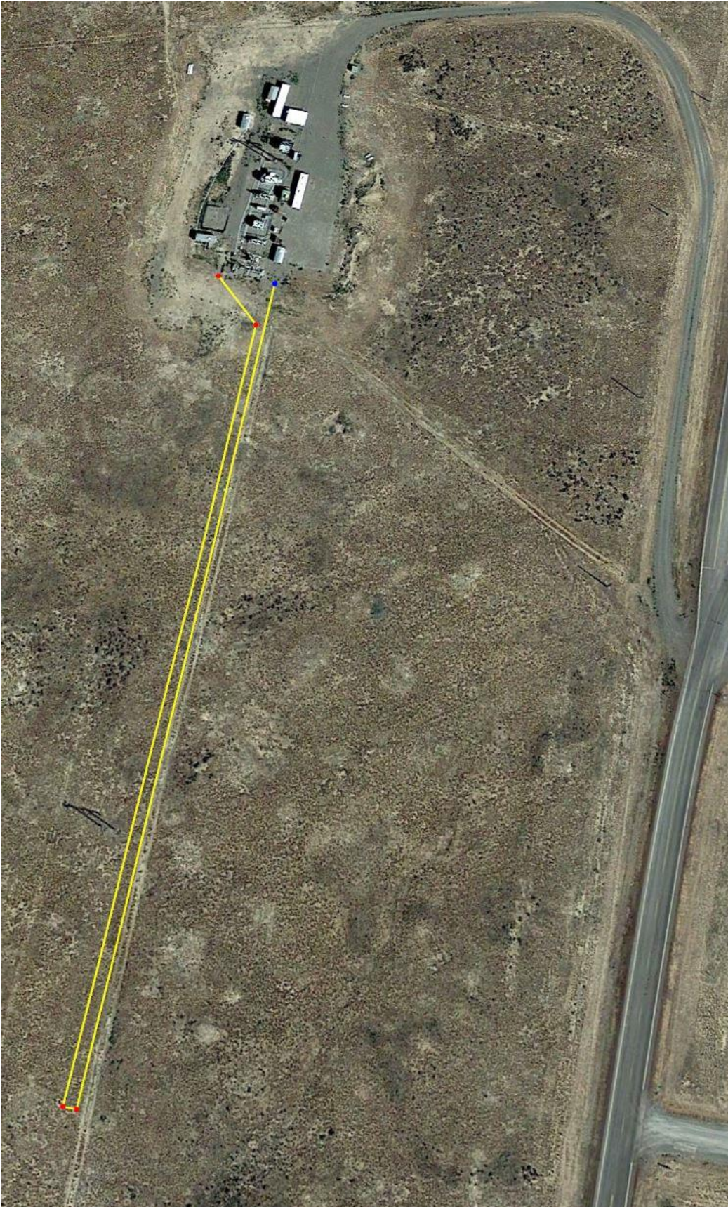
Figure 5: MFC Test Pad – 15kV cable layout
