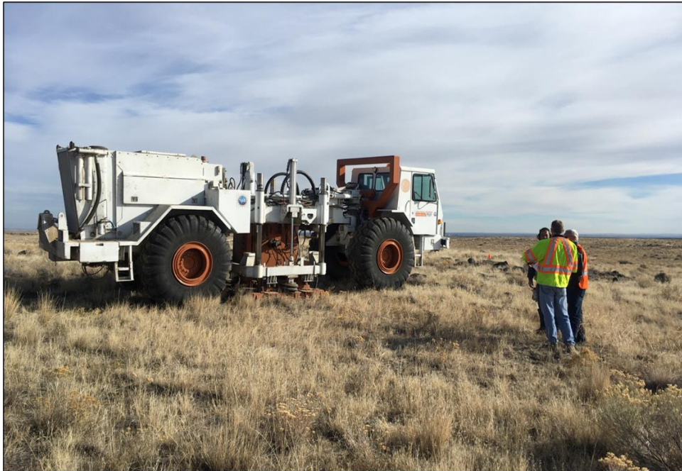
FIGURE 2. TRUCK-MOUNTED SURFACE WAVE SOURCE SYSTEM OPERATING AT THE CFPP IN OCTOBER 2019
