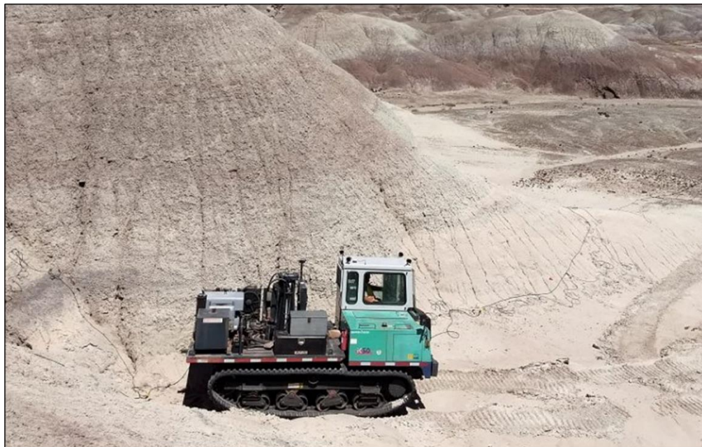
FIGURE 5. EXAMPLE FIELD DEPLOYMENT OF AN AF-450 HAMMER SYSTEM ON A RUBBER-TRACKED VEHICLE
