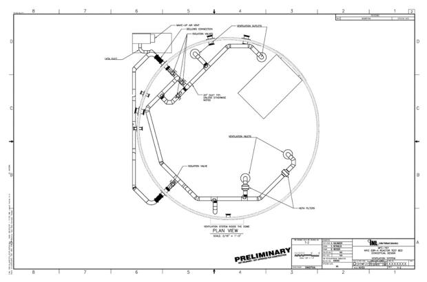
Figure 7. Ventilation system inside containment dome.
