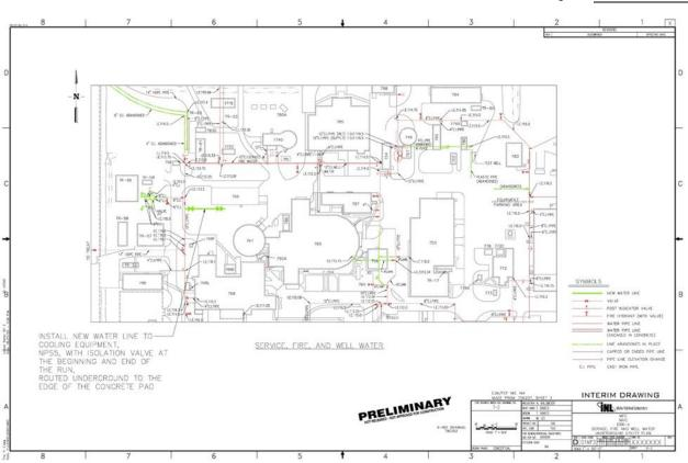
Figure 5. Underground utility plan.
