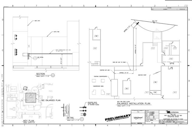
Figure 9. Compressed air routing from MFC-768 to the EBR-II dome.
