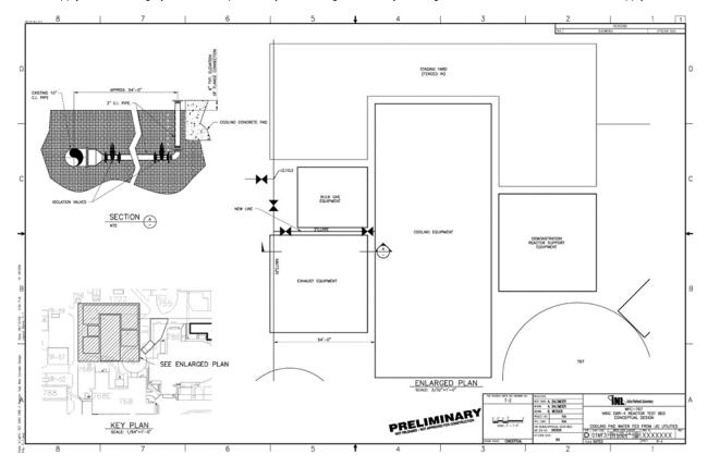
Figure 4. Cooling equipment water connection.
