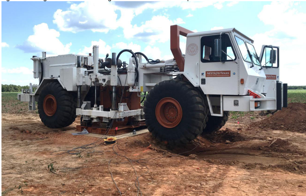
Figure R-6. Image shows surface wave generator truck and concrete pad with associated excavations.
