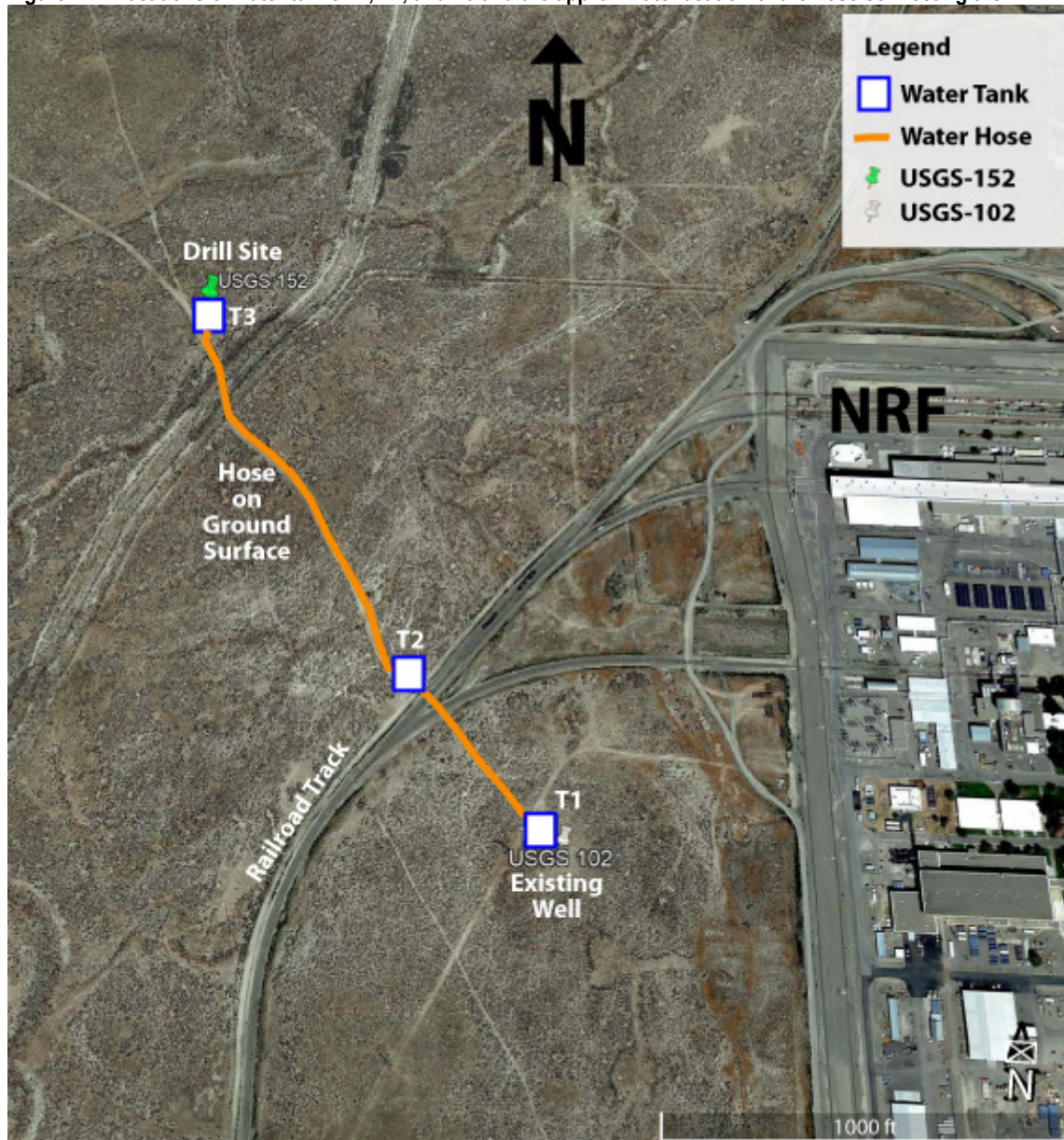
Figure R-7. Locations of water tanks T1, T2, and T3 and the approximate location of the hose connecting them.
