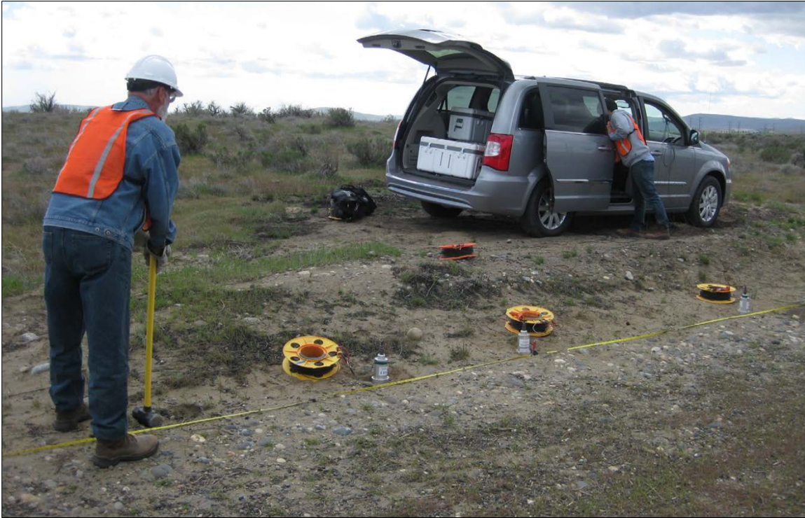
Figure 9. Example Geophone Receiver system to be employed during SASW surveys.
