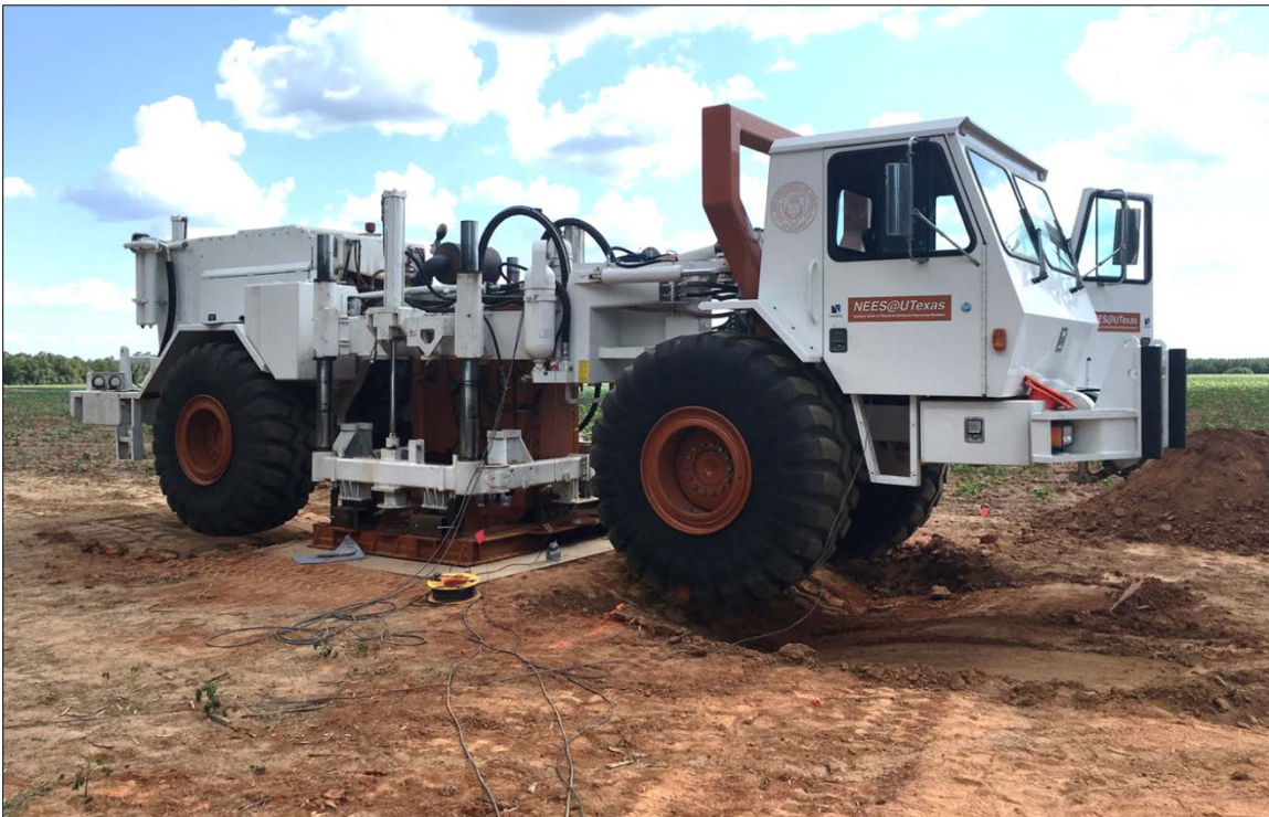
Figure 10. Example Field Deployment of the surface wave source system showing A concrete pad and excavations.
