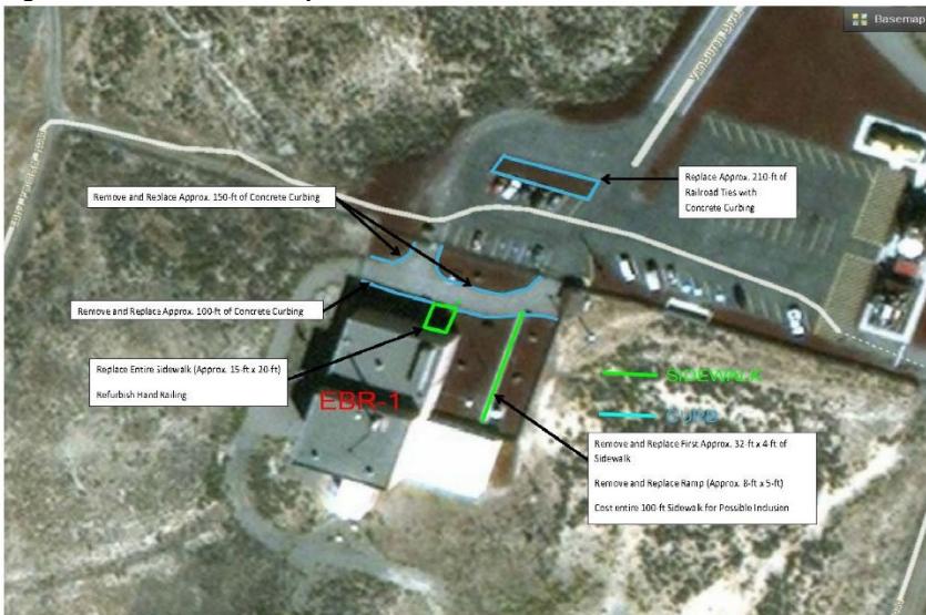
Figure 7. EBR-1 Concrete Improvements
