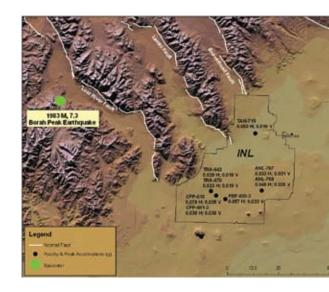
During the 1983 Borah Peak Earthquake, the Advanced Test Reactor only experienced a ground motion of 0.023g, or about 2 percent of the force of gravity. The reactor safely and automatically shut down. The ATR is designed to withstand ground motion of 0.24g.
