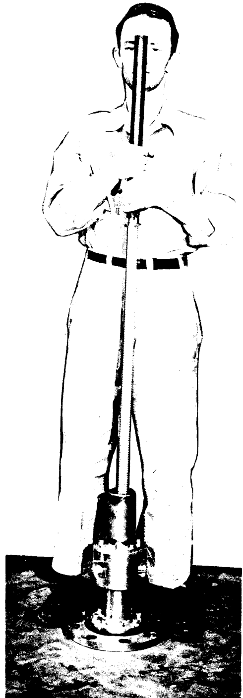
POSITION OF MECHANIC AFTER LIFTING CONTROL ROD 30 INCHES
