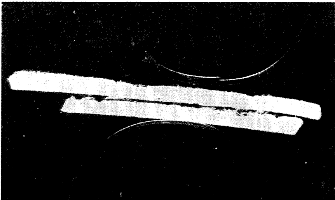
Figure I-43, Metallographic Samples #412 from Boron Strip #11, Fuel Element 60, Taken 3-1/2 Inches from the Top in a Non-Deteriorated Area.
