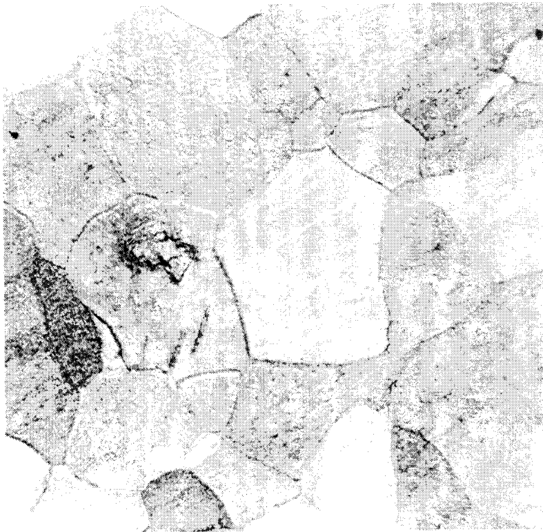
Figure I-61a, Structure of Cadmium at Top of Control Blade #1 Away from Weld. Transverse, 265x. Aqua Regia etch.
