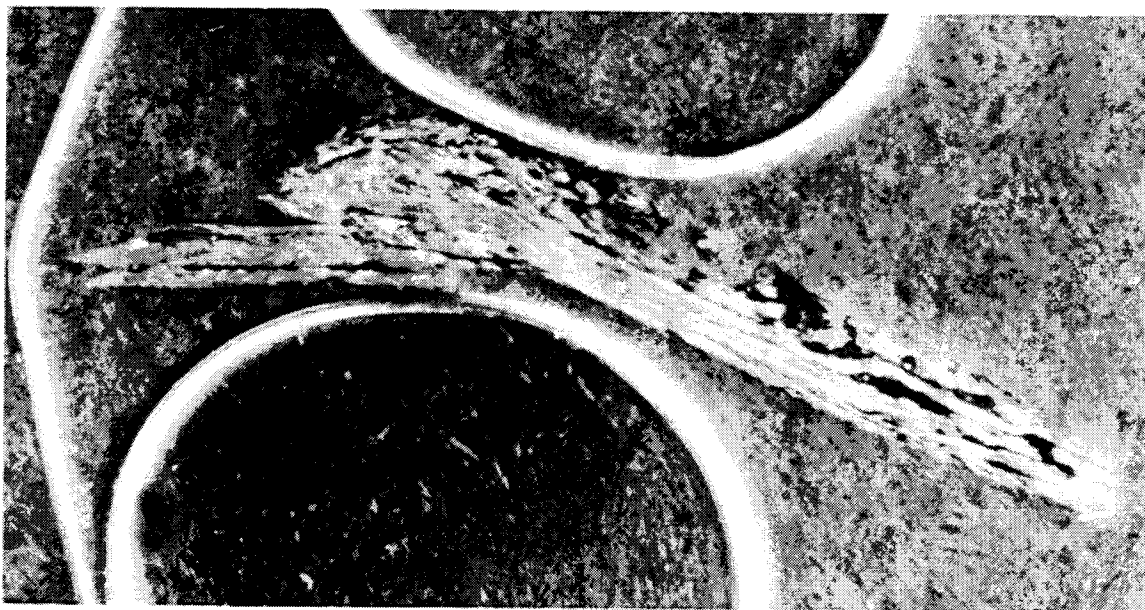
Figure I-48, Metallographic Samples #418 from Boron Strip #32, Fuel Element 50, Taken 11 Inches from the Top on the Highly Deteriorated Edge.
