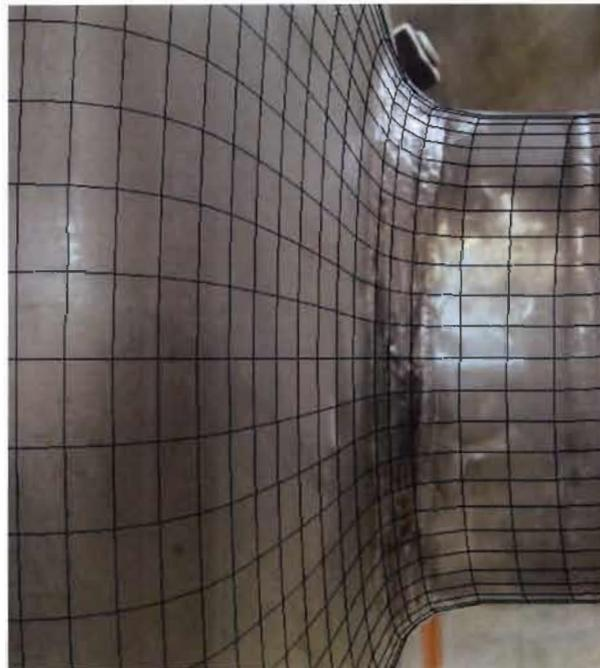
Figure F.2.5-4 – Cap mesh closely matches that of physical conditions, shown overlaid on picture.
