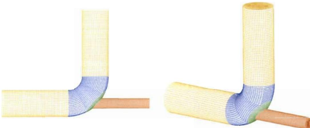
Figure F.1.1-2 – Quadrilateral shell mesh of the Pilot model’s unlisted branch component is shown.
