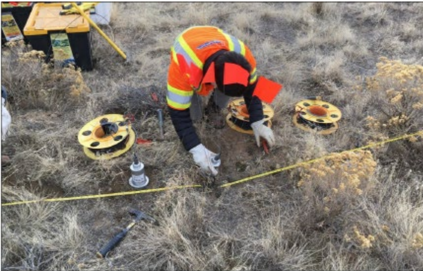
FIGURE 3. EXAMPLE GEOPHONE PLACEMENT ALONG ON AN SASW SURVEY LINE AT CFPP IN OCTOBER 2019
