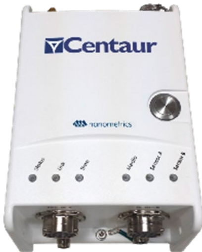
Figure 3. Nanometrics Centaur digitizer. This will digitize the data from the instruments and transmit the data via a 2.4 GHz radio.
