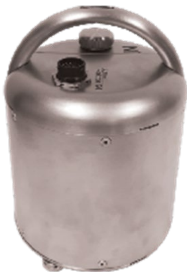
Figure 1. Titan SMA which will be used to measure ground acceleration.
