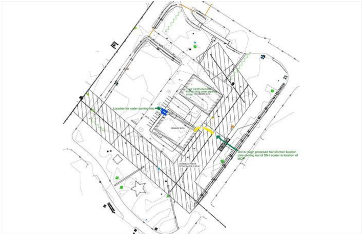
Figure 2. Site plan showing layout building locations and utility tie-in locations. Yellow represents the power connection. Blue indicates the location of the water connection.
