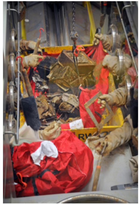
A protective glovebox allowed workers to sort through Pit 9 waste for repackaging.
