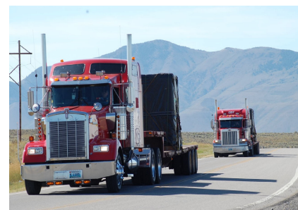
Concrete vaults moving to the Idaho Site's CERCLA Disposal Facility
